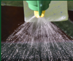
FAN AIR NOZZLES Standard on all booms, they reduce drift by up to 90%
